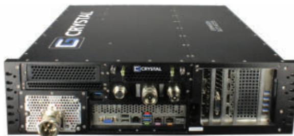
Crystal Group RS363S15F Rugged 3U Server with a depth under 15 inches
