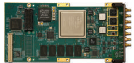
Pentek Jade Model 71141 6.4 GS/sec A/D and D/A XMC module for wideband defense, radar, and communication applications
